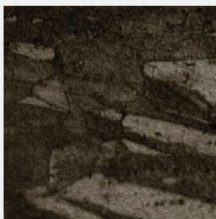
Conventional CuCrZr Grain Structure
